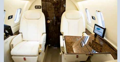
A SPACE NEW VIP SEATING FROM EXPERT DESIGNERS IACOBUCCI HE BOOSTS CABIN COMFORT AND USABILITY, DESIGNED TO MOVE FORE AND AFT AND SIDE TO SIDE, RECLINE FULLY, ROTATE 180°, AND ALLOW OCCUPANTS TO MAXIMIZE THEIR WOR-WORKING KING AND LIVING SPACE.
